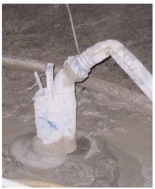
KTZ32.2 in use for drainage at the working face
